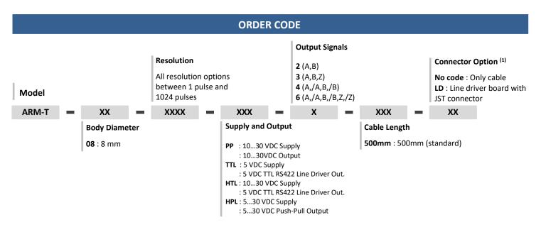
(1) If encoder is used only with cable; only A, B and Z output signals can be received. If encoder is used with line driver board with JST connector; A, /A, B, /B, Z and /Z output signals can be received.
