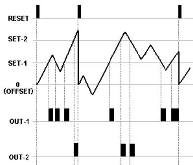
The outputs (TOUT) should be selected as a time in this mode. When the count value's each passing from the SET-1 value, OUT-1 gives an output in TOUT-1 time and stop, each passing the SET-2 value, OUT-2 gives an output and end of the TOUT-2 time it stop. When RESET comes, outputs and count value are reset.
