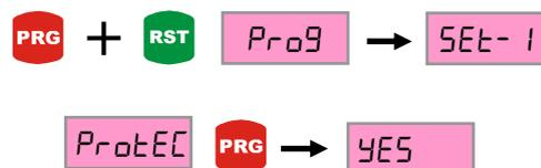
When press the PRG button selection flash on the display. Intended selection is set by UP-DOWN button. Press PRG button to save.
