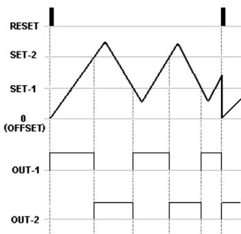
TOUT time should be selected as a HOLD. OUT-1 gives an output until the count value reach the SET-2 value and when it reach OUT-1 stop, OUT-2 start to pull. OUT-2 pulls until the count value reach the SET-1 value and when it reach OUT-2 stop and again OUT-1 pulls.
