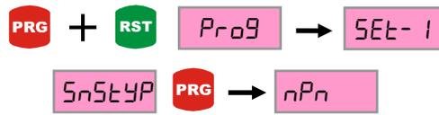
When press the PRG button selection flash on the display. Intended selection is set by UP-DOWN button. Press PRG button to save.
