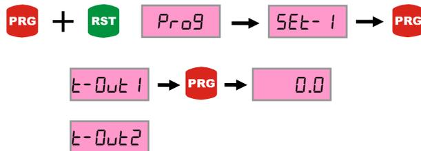
The right digit flash when press the PRG button on the display. The desired selection is set by UP-DOWN button. It is saved by pressing PRG button.
