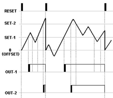
When count value rise from the SET-1, value OUT-1 gives an output and if it rise up from SET-2 value OUT-2 gives an output. Even it falls from the SET value ,relays do not stop until the RESET come, but when the RESET come it stops. If the time is entered for the outputs,relays gives an output and stop during this time,relays do not gives output until the RESET comes,even the fall or rise from the SET values.
