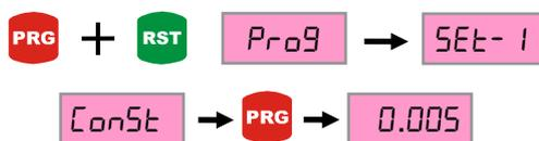
When press the PRG button, the right digit that is on the display flash. The intended value is set by UP-DOWN button. The digit shift to the left by using LEFT button. When press the PRG button the point flash. The point place is set by UP-DOWN button. Press PRG button to save.
