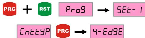
When press the PRG button selection flash on the display. Intended selection is set by UP-DOWN button. Press PRG button to save.
