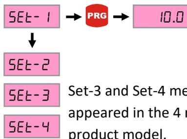
When press the PRG button the right digit flashing on display. Setting by UP-DOWN button. The digit shift to the leftside by pressing left button. Is saved by pressing the PRG button.
