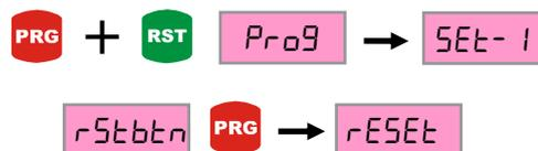
When press the PRG button selection flash on the display. Intended selection is set by UP-DOWN button. Press PRG button to save.
