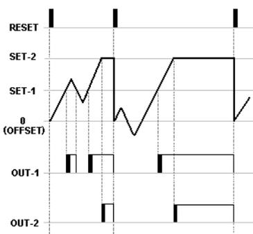
OUT-1 gives an output when the count value rise up to SET-1 and stop when it fall down. When rise up to SET-2 value OUT-2 gives an output and count value is fixed. Even the puls is come to device by encoder,count value is not changed without RESET coming, but when the RESET come, the count value and outputs are reset.
