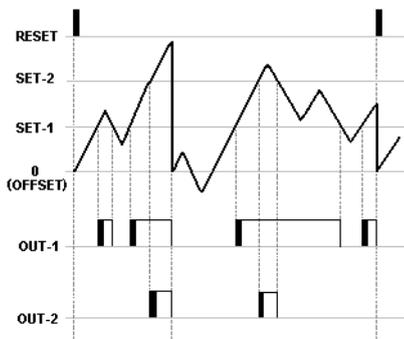
When the count value is over then the Set 1 value, OUT 1 gives an output in this mode (relay-1 pulls). If TOUT-1 (Relay-1 pull time) HOLD is selected, the OUT-1 will be held up to count value is below SET1. When count value exceed the SET-2 value OUT-2 gives an output and if TOUT-2 HOLD is selected the OUT-2 is held as a pulled until the count value fall down the SET-2. If TOUT-1 and TOUT-2 is selected with holding time, OUT-1 and OUT-2 will be held during setted holding time.
