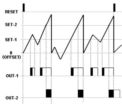
This is the Output-4 state that counting after the set-2 value. OUT-1 output is dependent on OUT-2. TOUT-2 should be selected with time. OUT-1 gives an output, the count value rise up to SET-1 value and it stop when it fall down, OUT-2 gives an output when it rise up to SET-2 value, End of the TOUT-2 time outputs and count value is reset automatically. Before the TOUT-2 time is not up, if RESET comes, the outputs and count number are reset.
