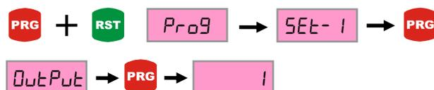
When the press PRG button in the selection display the right digit flash. The desired selection is set by using UP-DOWN button. It is saved by pressing PRG button.
