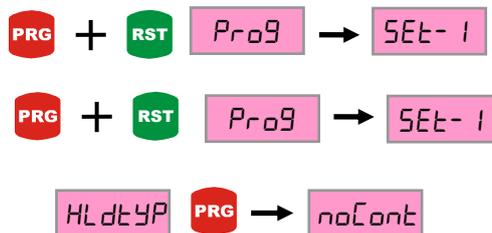
When press the PRG button selection flash on the display. Intended selection is set by UP-DOWN button. Press PRG button to save.
