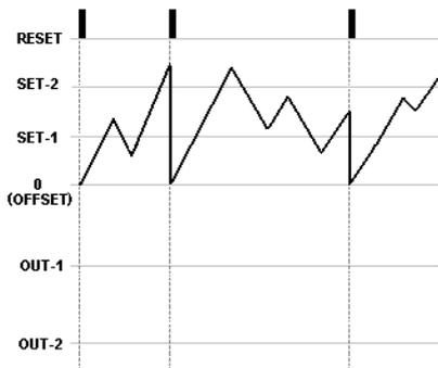
When the Out mode is selected 0, Out-1 and Out-2 do not give any output.
