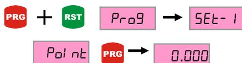
When press the PRG button, the right digit that is on the display flash. The intended value is set by UP-DOWN button. The digit is shifted to the left side by pressing the left button. Press PRG button to save.
