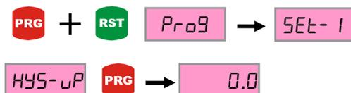
The right digit flashed by pressing the PRG button on the display. Intended value is set by UP-DOWN button. The digit shift to the left side by using the left button. The value is saved by pressing PRG button.
